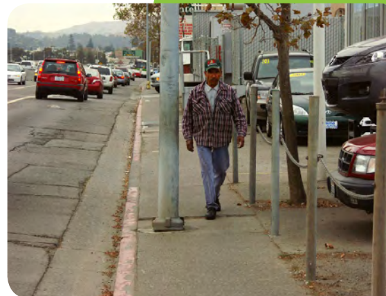
Lamp posts, hydrants, trees and other objects further reduce the usable sidewalk width.
