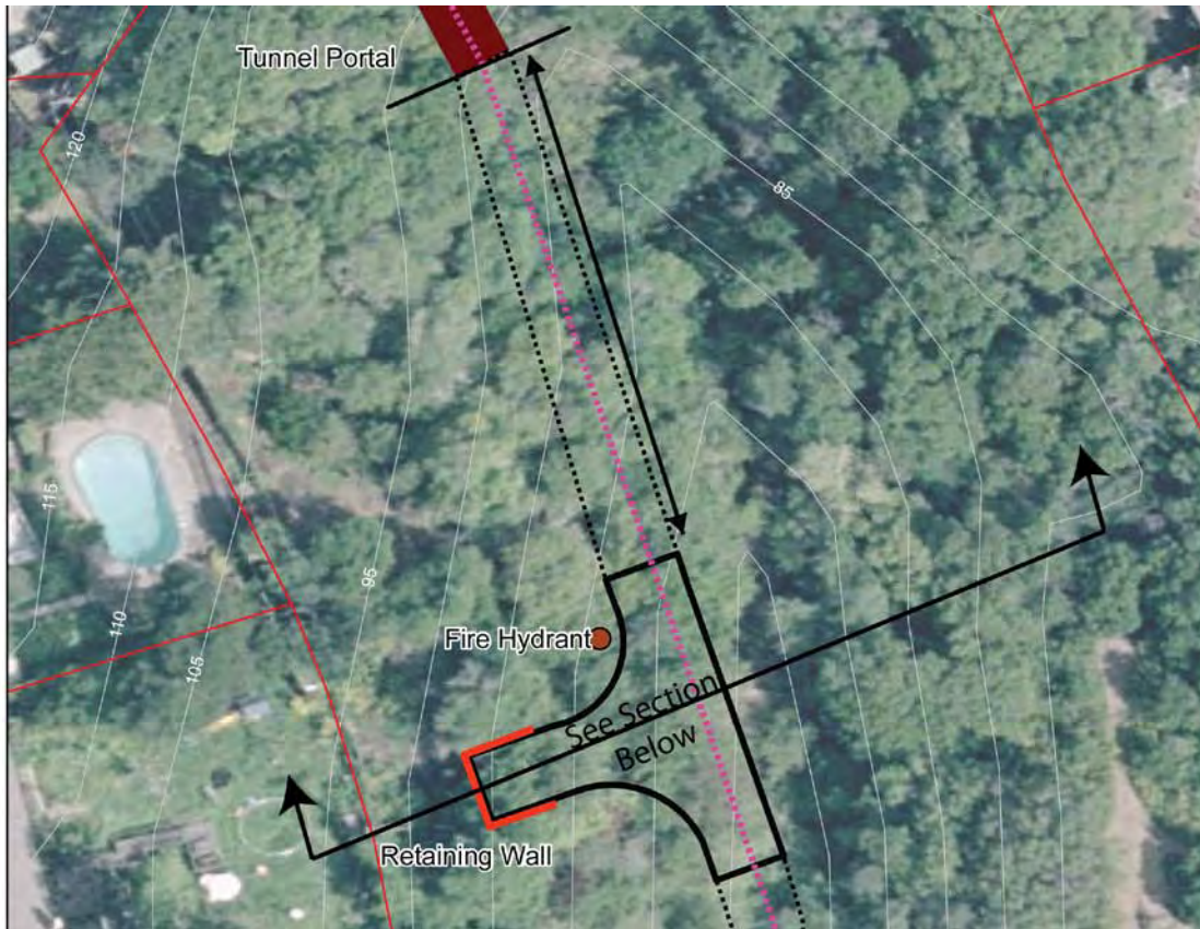
Figure 2-24: South Portal Emergency Vehicle Turnaround Plan
