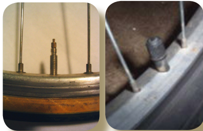
Left: Presta valve, Right: Schrader valve
